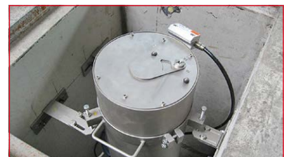
IR camera in a special protective housing for measuring after pressing
